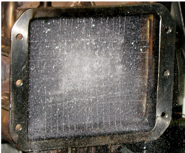
Figure 6. Flow Visualization of Pulsejet Fuel Injection
